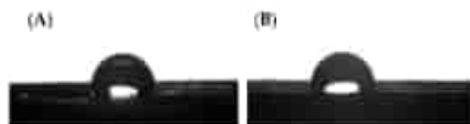
Figure 17. Droplets applied on the bottom part of the dumbbells for samples containing 20% vol. (A) with non-degassed base diatomite, and (B) with non-degassed fractionated diatomite.
